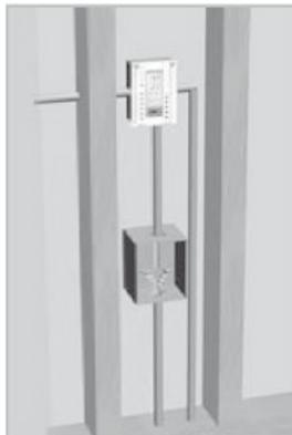
4 Connect the floor temperature safety sensor to the thermostat through a conduit, and install between two heating ribbons, at least 50 cm from the wall.
